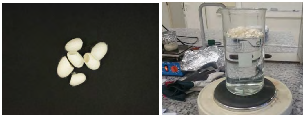
Fig 5. Silk cocoons(left); degumming of silk cocoons (right).
