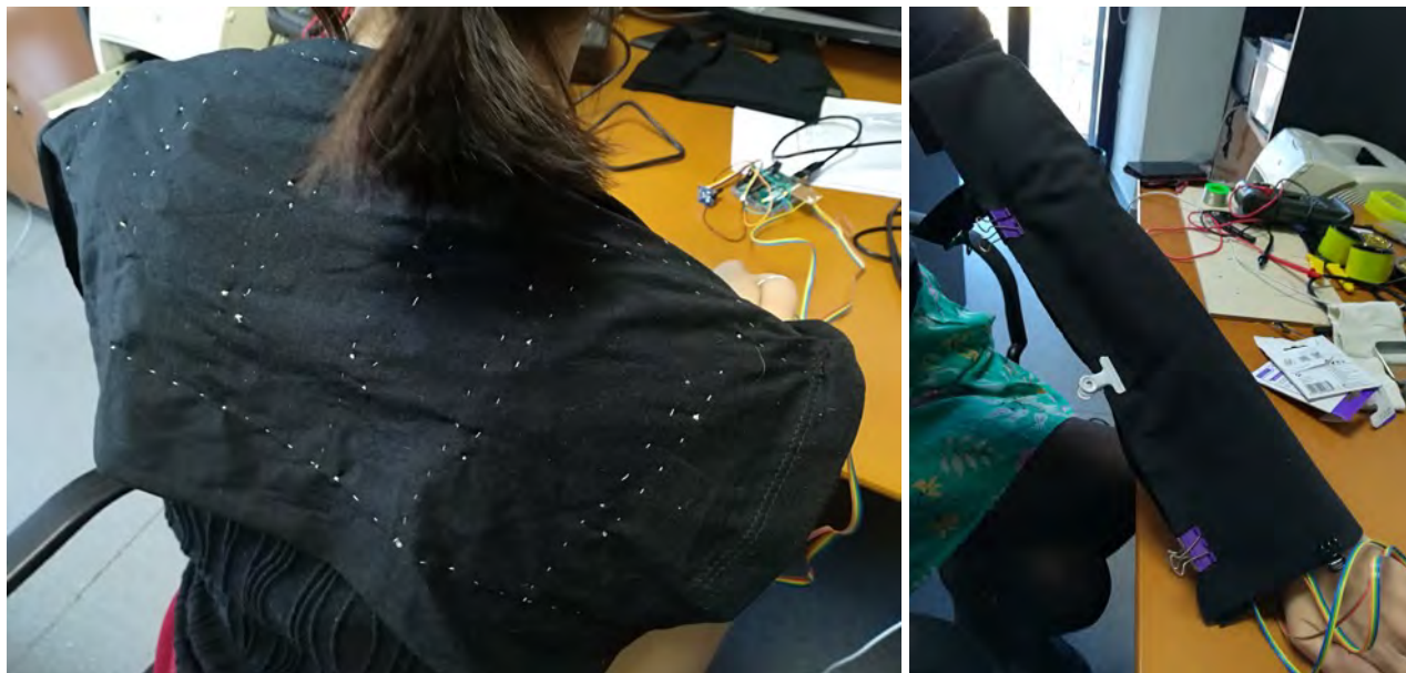
Fig 3. The second prototype of Magic Lining allows the user to sense vibration movements from one end to another, inside out and outside in, on the back and around the arm.
