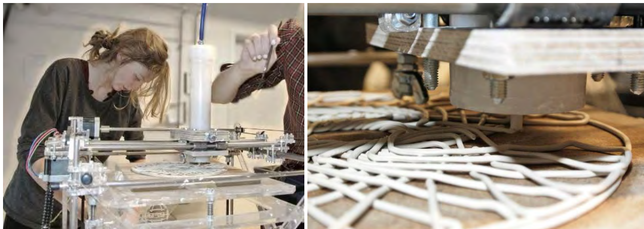
Fig 2. Left: The RapMan utilized for 3d printing with clay. Right: the very genesis of shape in 3d printing: the extrusion of a line of material.
