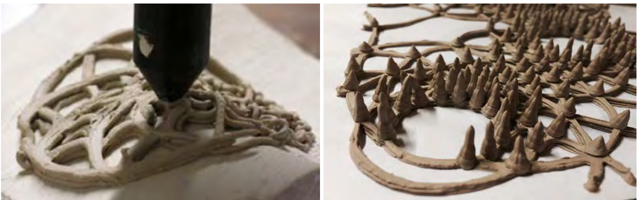
Fig 5. Left: Test of "overforming" by robotic 3D printing with porcelain upon the hand-modelled mould. Right: Test of plasticity and "life" of clay expressed through spikes.
