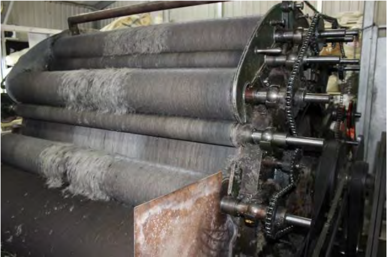
Fig 7. The mixed composition recycled materials being carded on a wool carding machine.
