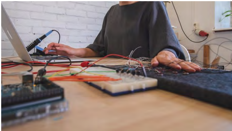
Fig 4. The third prototype of Magic Lining allows the user to sense vibration movements under his/her hand. The aim is to create body sensations that relate to materials.
