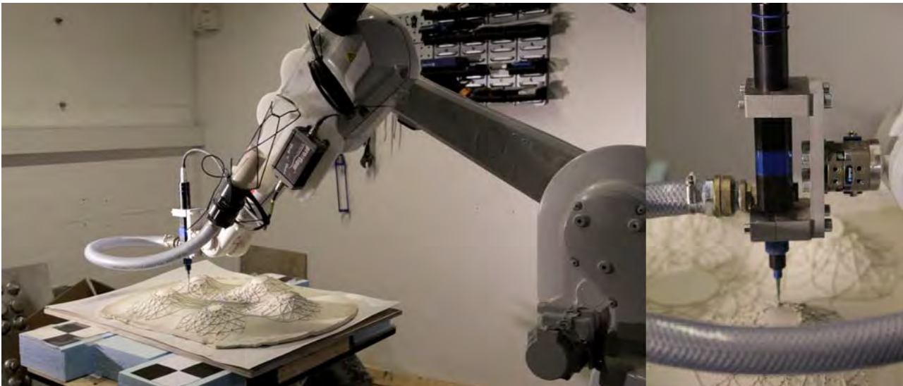
Fig 9. The adapted 3d printed paths are driving the robotic movement of a clay extruder nozzle with porcelain that prints on the top of the hand modelled mould.
