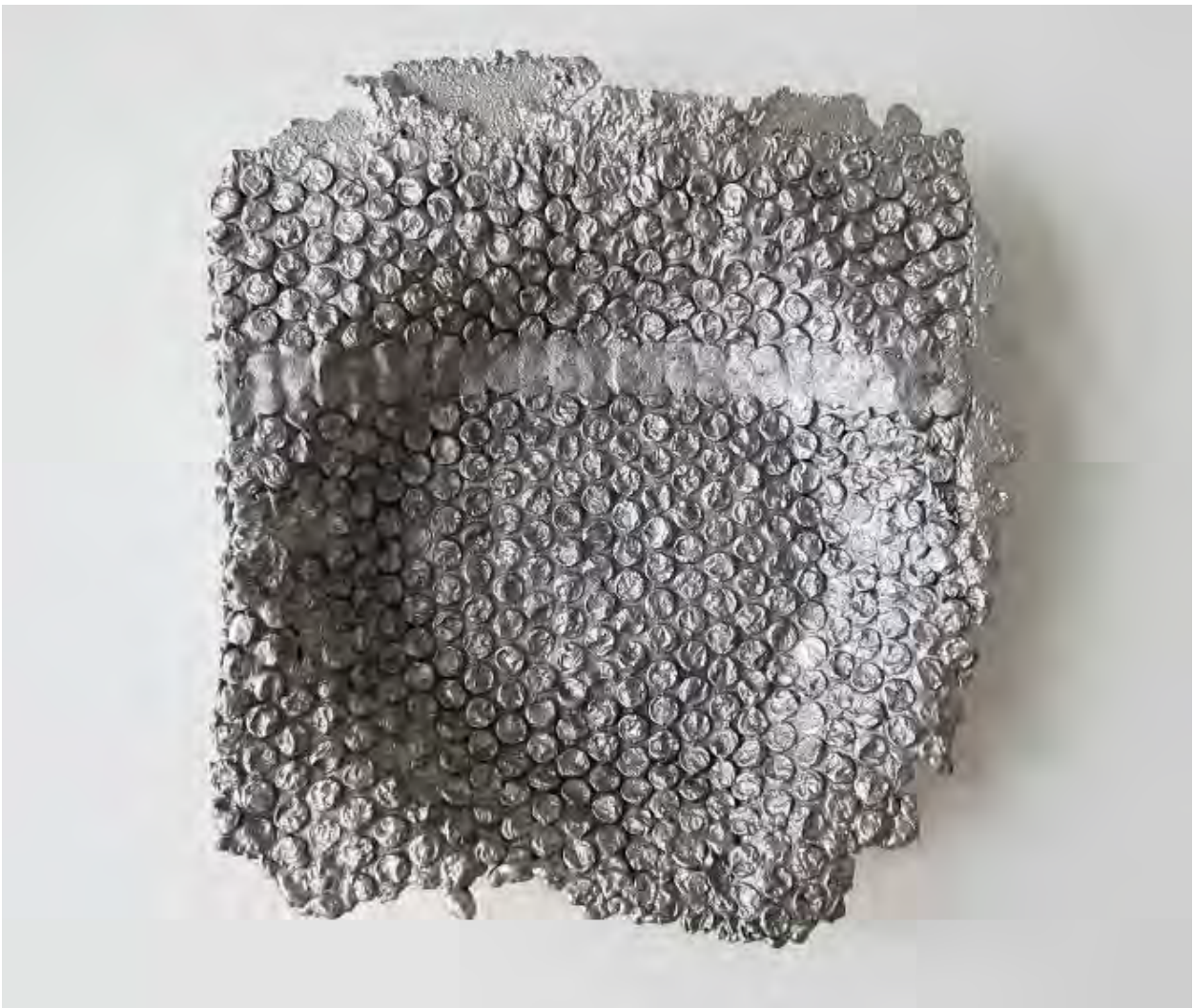
Fig 1. Sand cast aluminium bowl using bubble wrap as a waste mould (Lambert, 2015).
