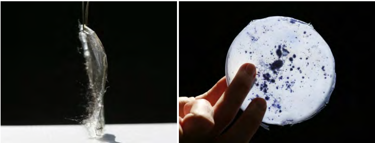
Fig 13. Film composite with stainless steel fibre (left); silk film with heat sensitive pigment (left).
