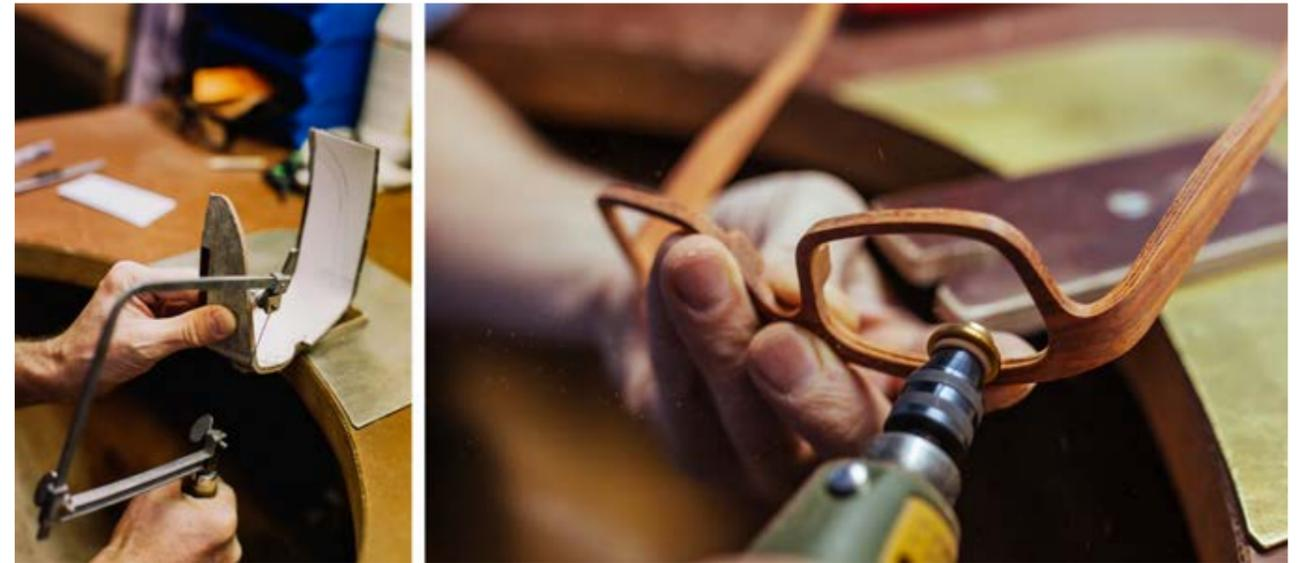
Process of making a wooden frame.
